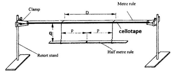
Note that the distance p is measured from the centre of the half-metre rule
