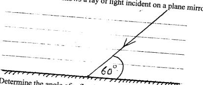
Determine the angle of reflection when the mirror is rotated 10° anticlockwise
