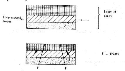
Two parallel lines of weakness develop and these form reverse faults.
