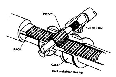
The rack consists of a cylindrical steel bar which has gear teeth machined on one side. The steel pinion, which is attached to the lower end of the steering column, is meshed with the teeth of the rack. When the steering wheel is rotated, it causes the rack to move to and fro along its axis. The ends of the rack are connected to the steering track arms by the short balt jointed tie rod ends. Therefore, its movement causes the wheels to turn through this mechanism.
