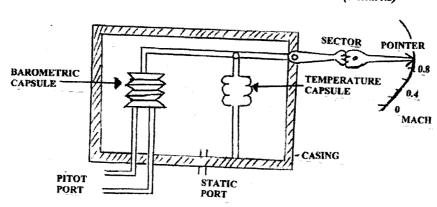
When the aircraft is stationary the capsule pressure and casing pressure are equal and the instrument reads zero. When the aircraft moves forward the pitot pressure increases because of ram effect for the capsule pressure to overcome casing pressure to expand the capsule.
