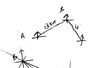
23. Three villages A B and C are such that B is 13 km on a hearing of 030° from A. C is 4km on a hearing of 120° from B.
