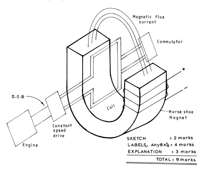
The aircraft engine rotates through a constant speed and drives a coil placed in a strong magnetic field.
