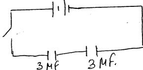
Determine the charge stored in the combined capacitance when the switch is closed. (3mks
