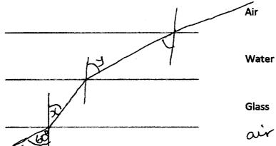
Given that the refractive indices of glass and water are  $\frac{3}{2}$  and  $\frac{4}{3}$  respectively. Calculate i) The angles X and Y (2mks
