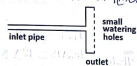
b. The diagram below shows a device used for watering crops out let has N number of holes. Inlet has a cross-section area of 2.4cm<sup>2</sup> and water flows at 15m/s. calculate the number of small holes if each hole has a cross-section area of 3mm<sup>2</sup> and water come out at 25m/s. (3 mark)
