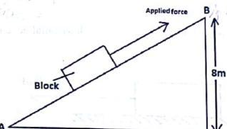
If distance AB is 25m and work done against friction is 240J calculate the value of applied force (3 mark)
