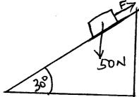
Determine the force required to move the body up the incline with constant velocity.
