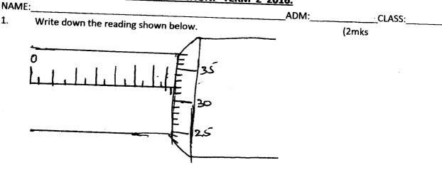
If the instrument has a zero error of -0.02mpletermine the actual reading of the measurement. b. (2mks
