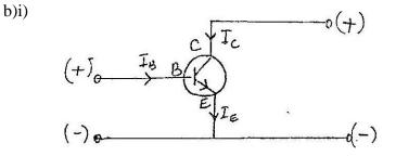
ii)  $I_B = {}_{0.5/100} x 2 = 0.01 mA$  $I_E = I_C + I_{rs}$   $I_C = 2-0.01 = 1/99MA$
