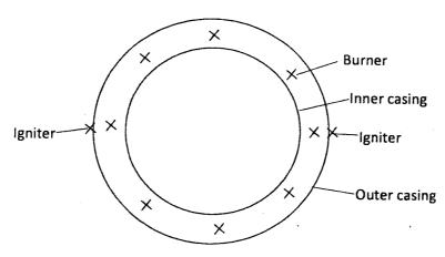
This type of combustion chamber consists of a single flame tube completely annular in form, which is contained in an inner and outer casing. The burners are suspended in the annular for supplying the fuel from the fuel manifold. There are two igniter plugs, one on each side of the engine.
