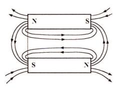
Correct polarity on each magnet
