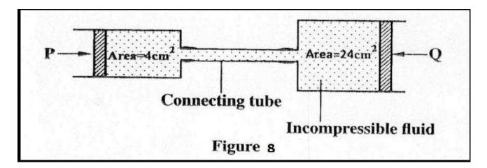
Opposing forces P and Q are applied to the pistons such that the pistons do not move. If the pressure on the smaller piston is 5 N cm2, Determine force Q. (2 marks)
