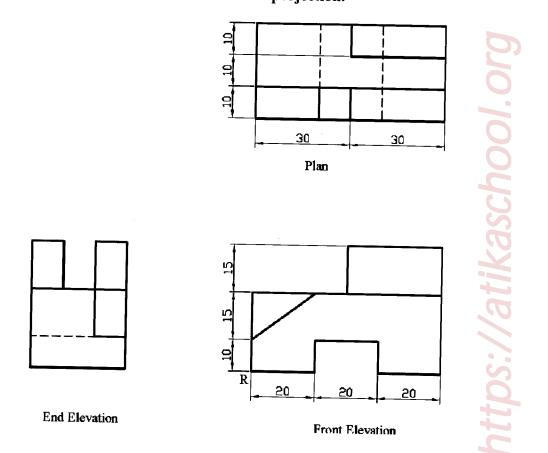
To a scale of 2:1, draw the block in isometric projection taking R as the lowest point.
