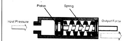
These activators work hydraulically in one direction only. They require a mechanical force to return them to the original position. Mostly the single acting activator makes use of a spring force.
