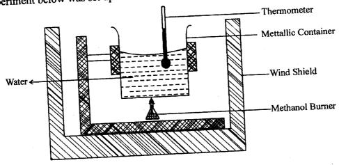
The following data was obtained from the above experiment. 62.74g Mass of burner + methanol before burning 62.36g Mass of burner + methanol after burning 38.5°C Final temperature of water 23.5°C
