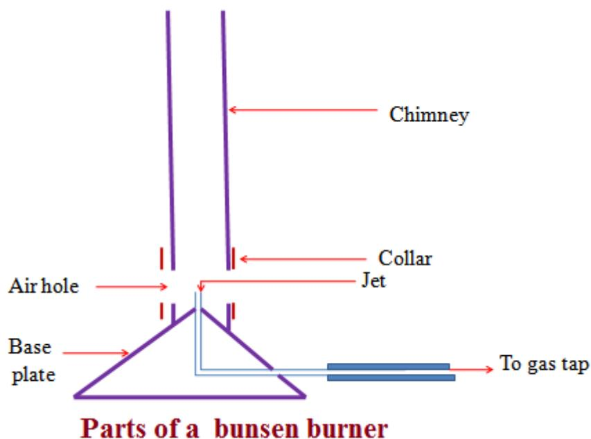
A Bunsen burner uses butane/laboratory gas as the fuel. The butane/laboratory gas is highly flammable and thus usually stored safely in a secure chamber outside Chemistry school laboratory. It is tapped and distributed into the laboratory through gas pipes.
