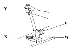
Which pair of the positions V, W, X and Y represents the load and pivot?
