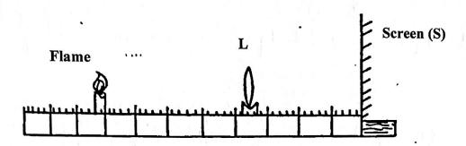
i) Describe how the set up may be used to determine the focal length f, of the lens. (3 marks)
