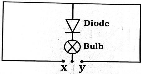
When switch is closed at x, the lamp lights but when switch is closed at Y, the lamp does not light. Explain this observation. (2 marks)
