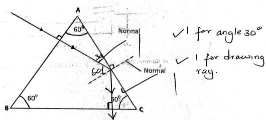
Sketch the path of the ray as it travels from face AC. (critical angle for glass is  $42^0$ ) (2 marks)
