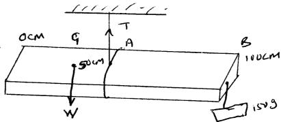
3. A uniform metre rule of uniform width 2.5cm and thickness 0.5cm is suspended at 80cm mark and kept balanced by hanging a mass of 150g at 100cm mark as shown below.
