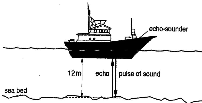
The sea bed is 12 m below the echo-sounder. Given that the speed of sound in water is 1300m/s to calculate the time between the sending out of the pulse and receiving its echo. (3marks)
