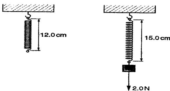
With no load, the spring is 12.0 cm long. With a load of 2.0 N on the end of the spring, its length is 15.0 cm. Calculate the spring constant (3 marks)
