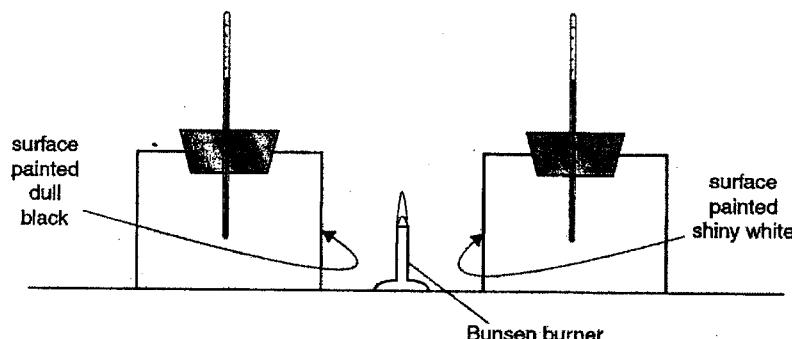
The containers, which are identical, are painted on the outside. One is dull black, the other is shiny white. Both are filled with water, initially at the same temperature. A Bunsen burner is placed equidistant between the cans as shown and left on for 30min. On the axes below sketch graphs to show the variation of temperature with time for the two surfaces (2marks)
