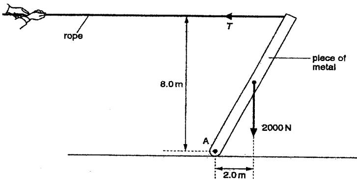
A man pulls on the rope with a horizontal force  $T$ . The piece of metal has a weight of 2000 N and is freely pivoted at A. The system is in equilibrium. By taking moments about A, calculate  $T$ . (3 marks)
