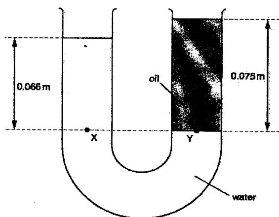
Points X and Y are at the same horizontal level. X is 0.066 m below the top surface of the water. Y is 0.075 m below the top surface of the oil. The pressure caused by 0.066 m of water at X is equal to that caused by 0.075 m of the oil at Y. Determine the density of the oil. (3marks)
