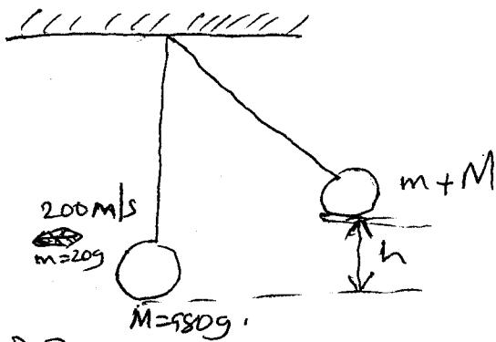
a) The velocity of the bullet and block immediately after collision (3mks)
