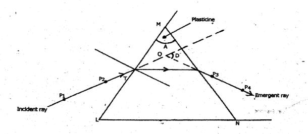
ii) Measure angle A of the prism using a protractor A=....
